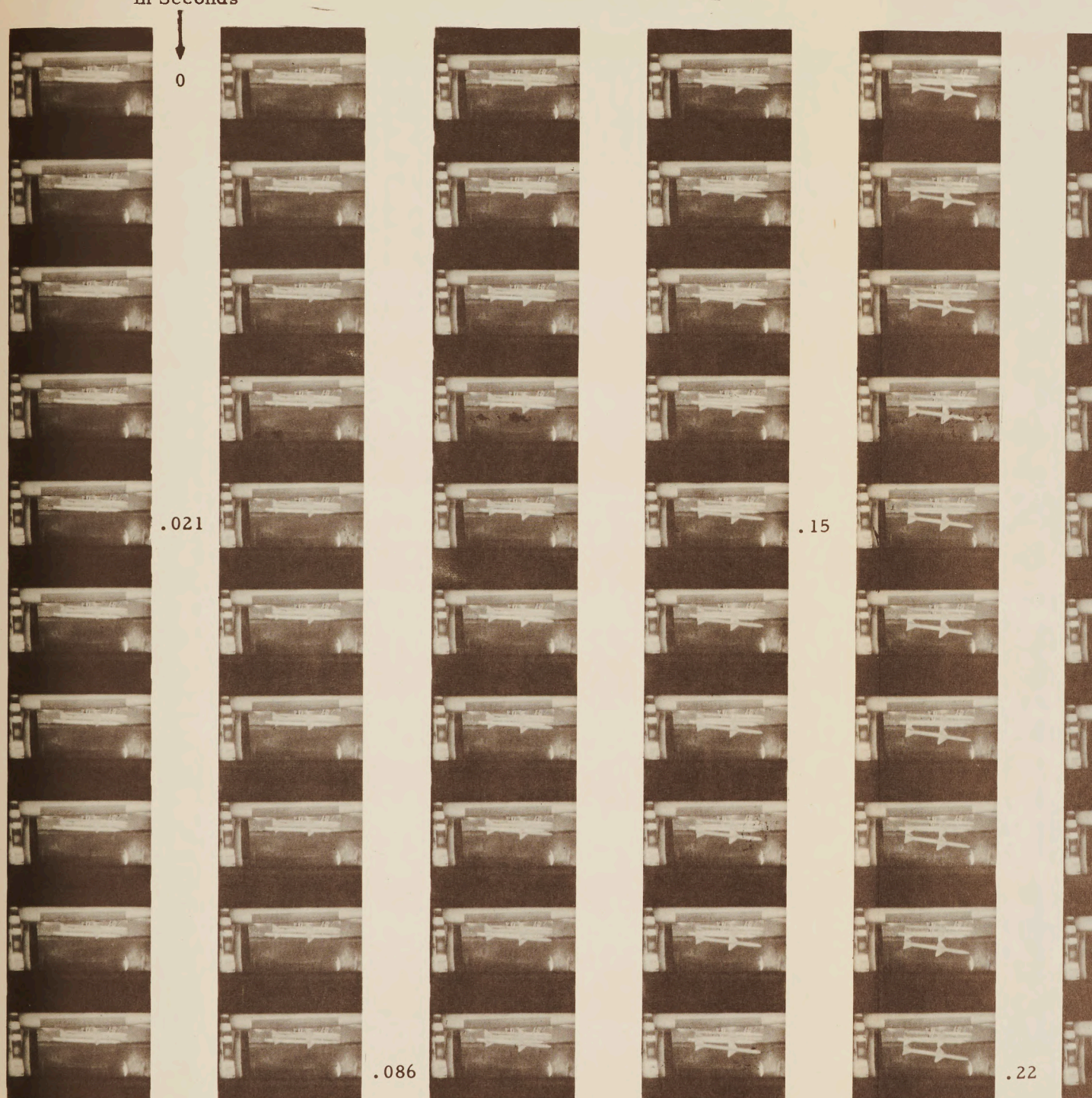
FIG. 14 (b) SIDE VIEW RUN NO.54 - SEA LEVEL, M = .8 , \alpha = 1^\circ , CONFIGURATION 2, \psi = 5^\circ FILM SPEED 880 frames per second
