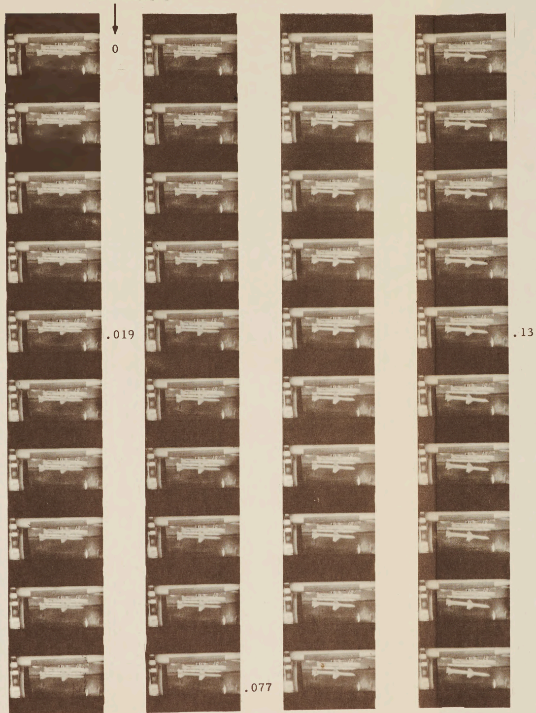
FIG. 12 (b) SIDE VIEW RUN NO. 47 - SEA LEVEL, M = .8 , \alpha = 1^\circ CONFIGURATION 1, \psi = 5^\circ FILM SPEED 980 frames per second
